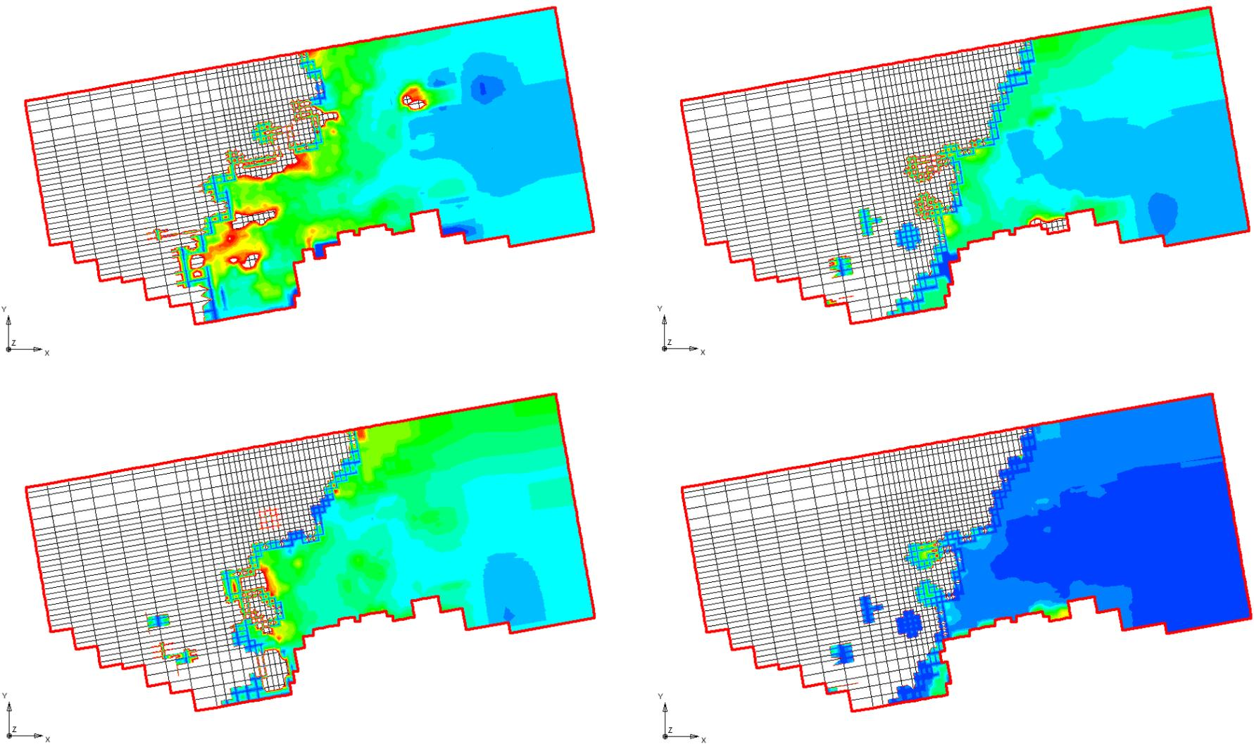
Figure 2: Distribution of vertical leakance between model layers: layer 1 to 2 - upper-left, layer 2 to 3 – lower left, layer 3 to 4 – upper right, layer 4 to 5 – lower right.
