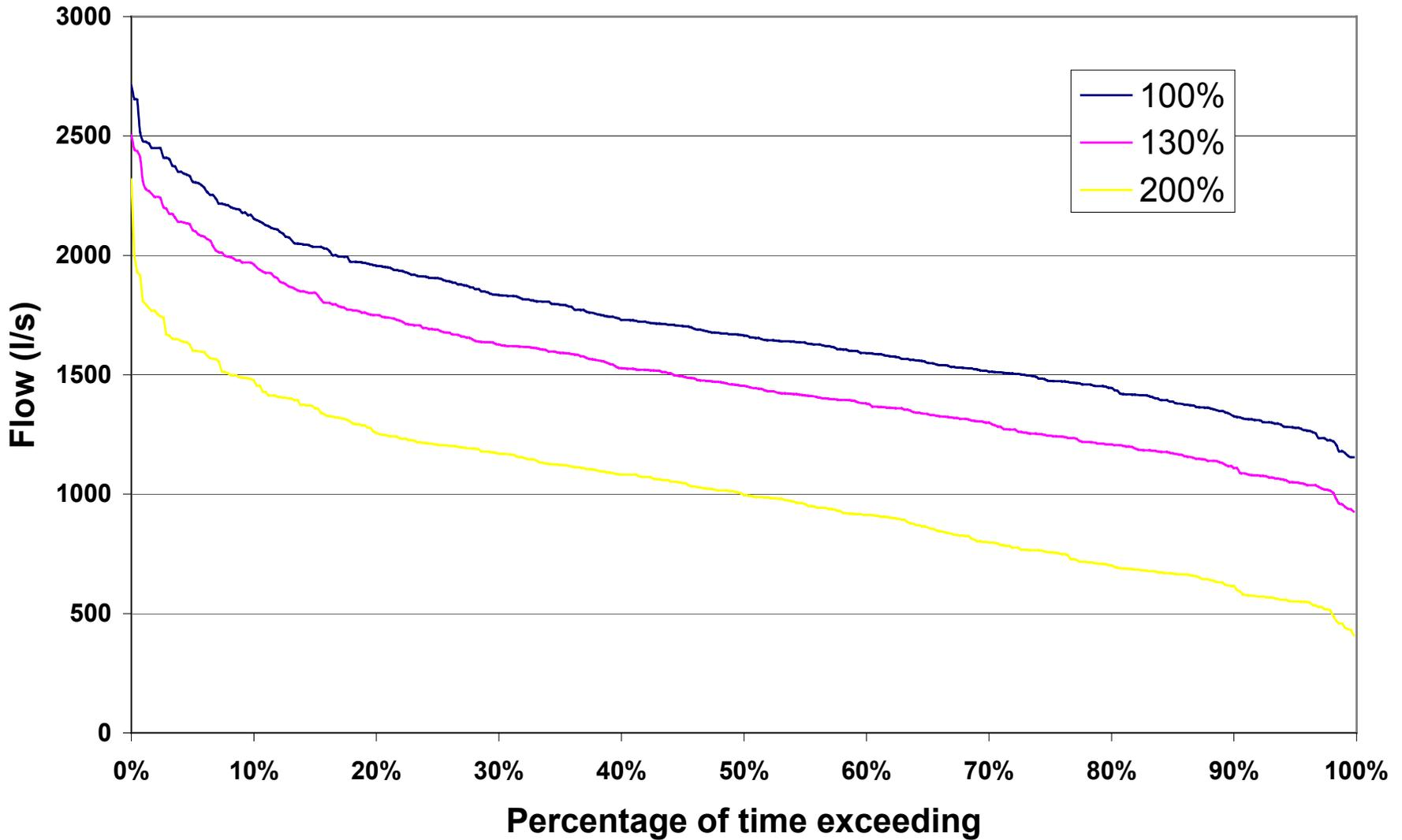
Figure 9: Distribution of simulated Avon River baseflow for groundwater abstractions of 100%, 130% and 200% of 1998/99 rate.
