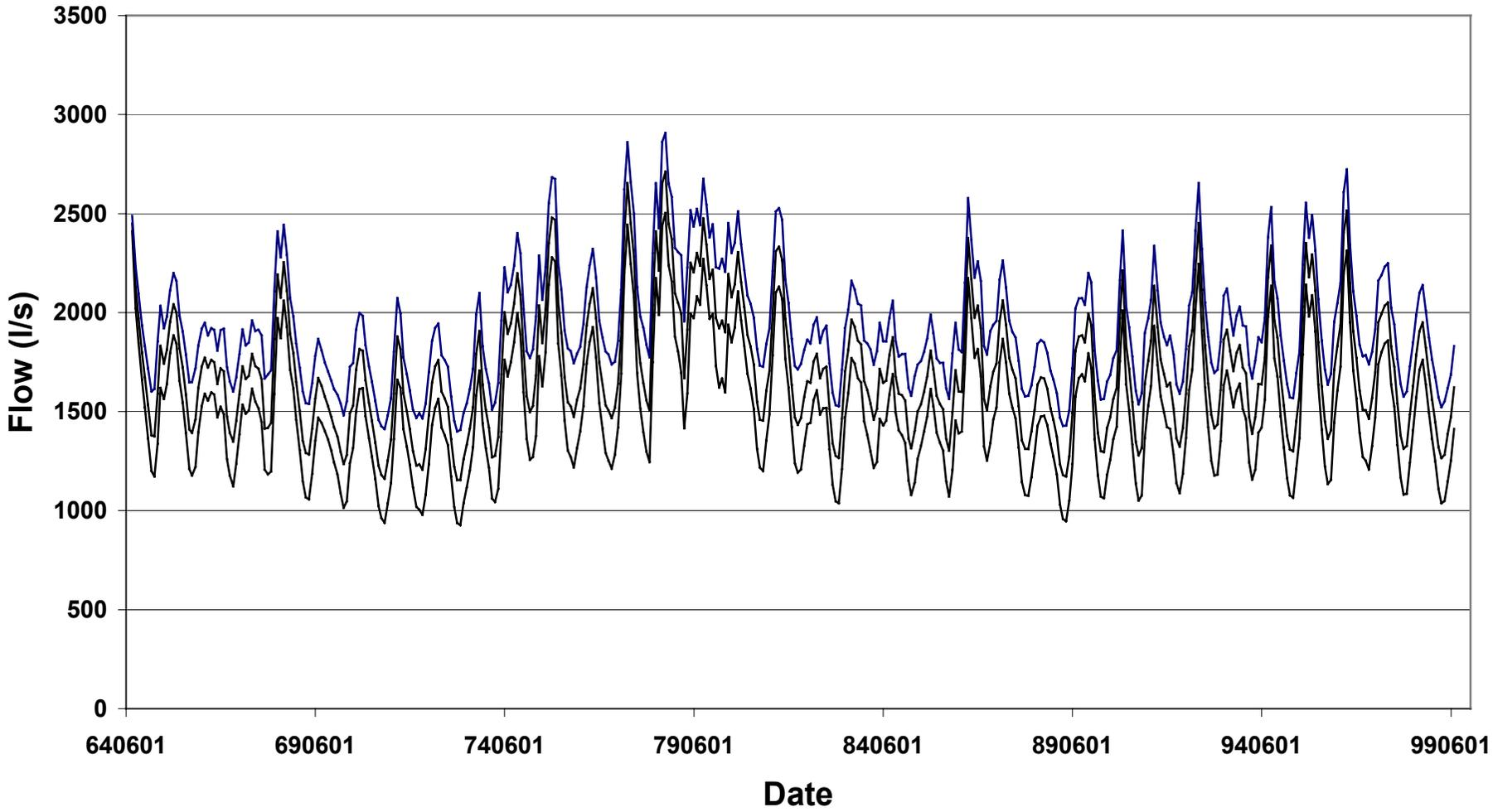
Figure 8: Simulated Avon River baseflow for groundwater abstractions of 70%, 100% and 130% of the 1998/99 rate.
