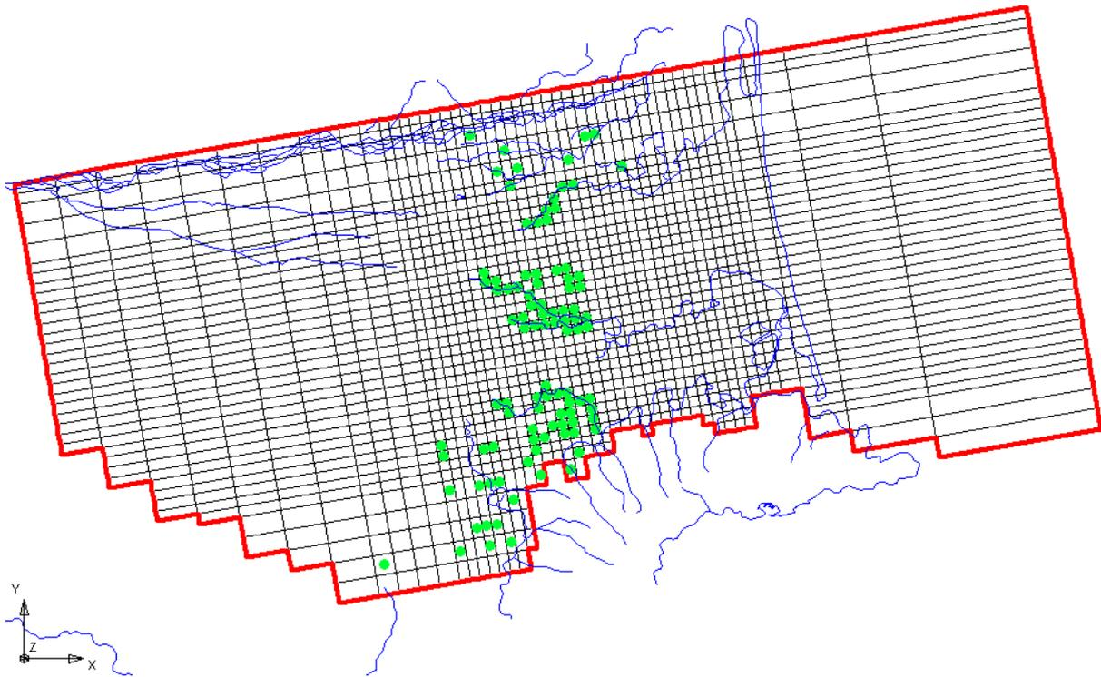
**Figure 5: Configuration of drain cells representing groundwater inflow.**
