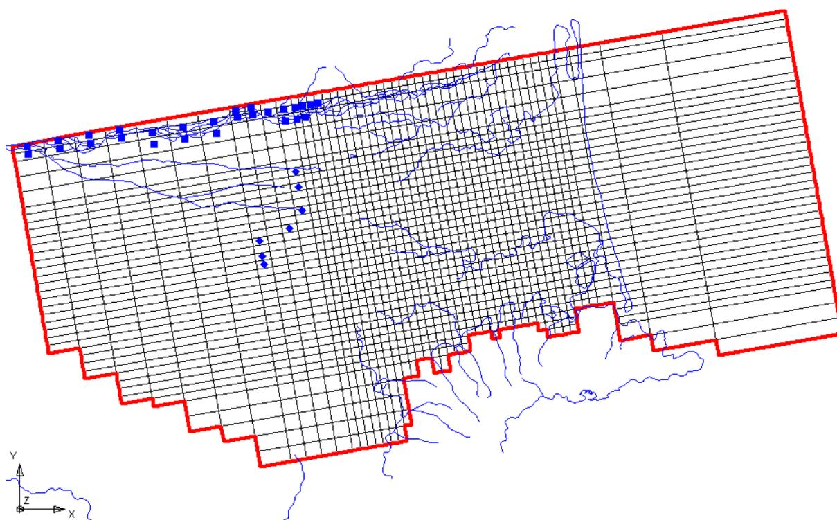
**Figure 3: Location of model river cells (■) and recharge wells (♦) shown in relation to surface water features.**
