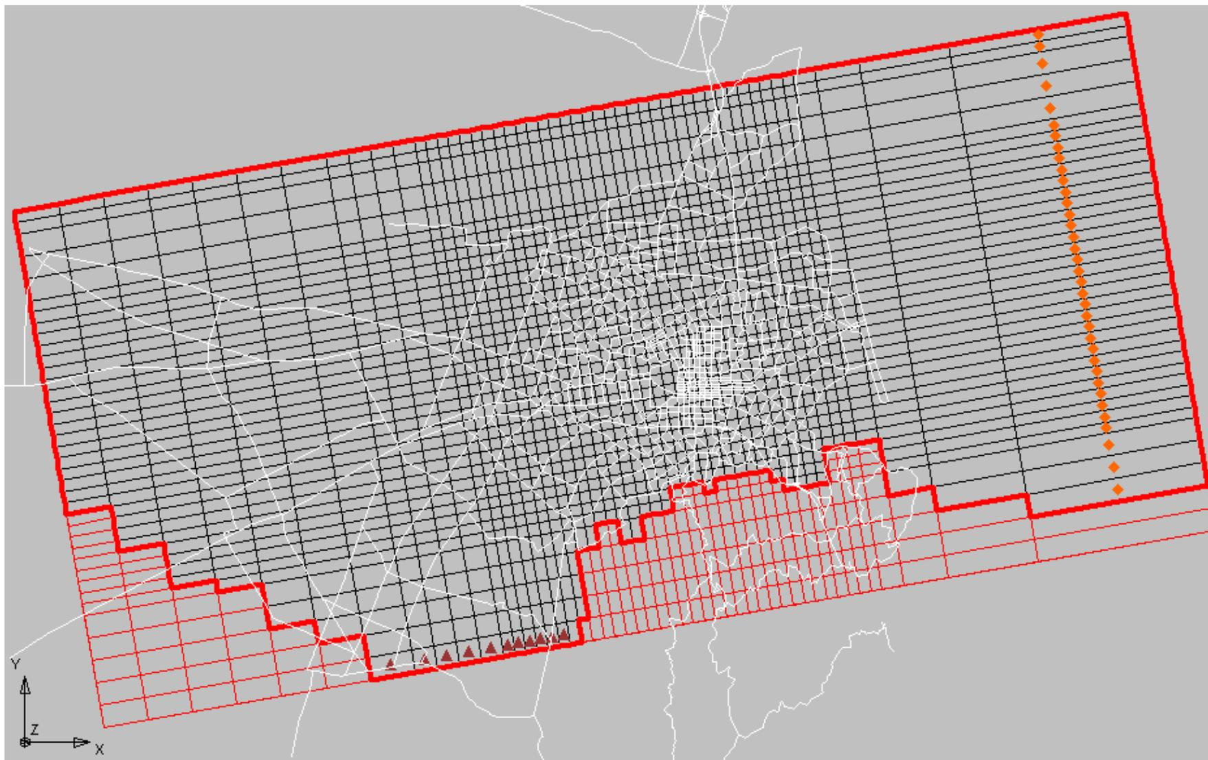
**Figure 1: Extent and boundary conditions of the Christchurch - West Melton groundwater model.**
