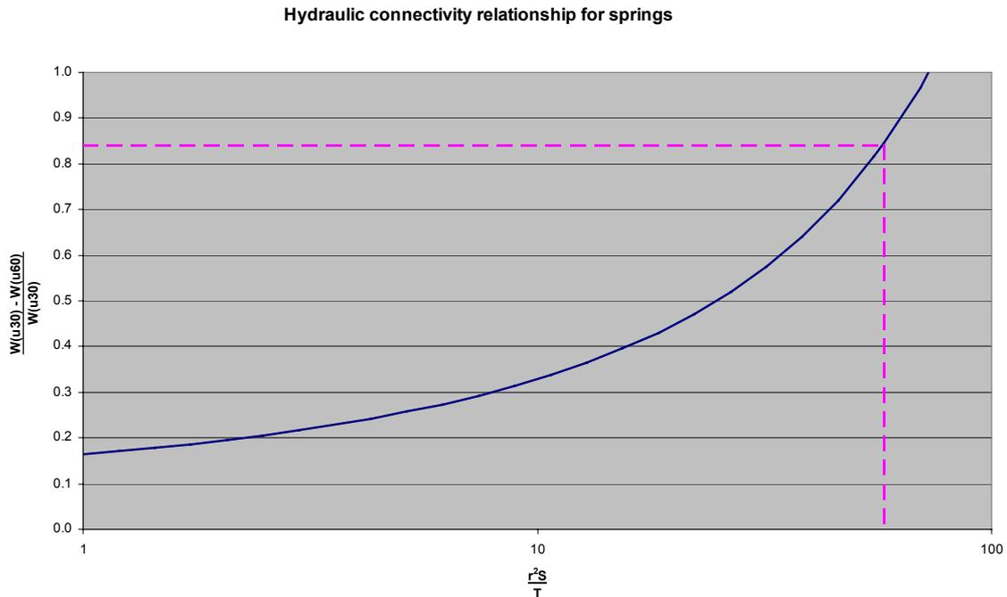
**Figure A2-3: Degree of hydraulic connection of a well and spring expressed in terms of the residual effect after 30 days pumping and 30 days shutdown.**
