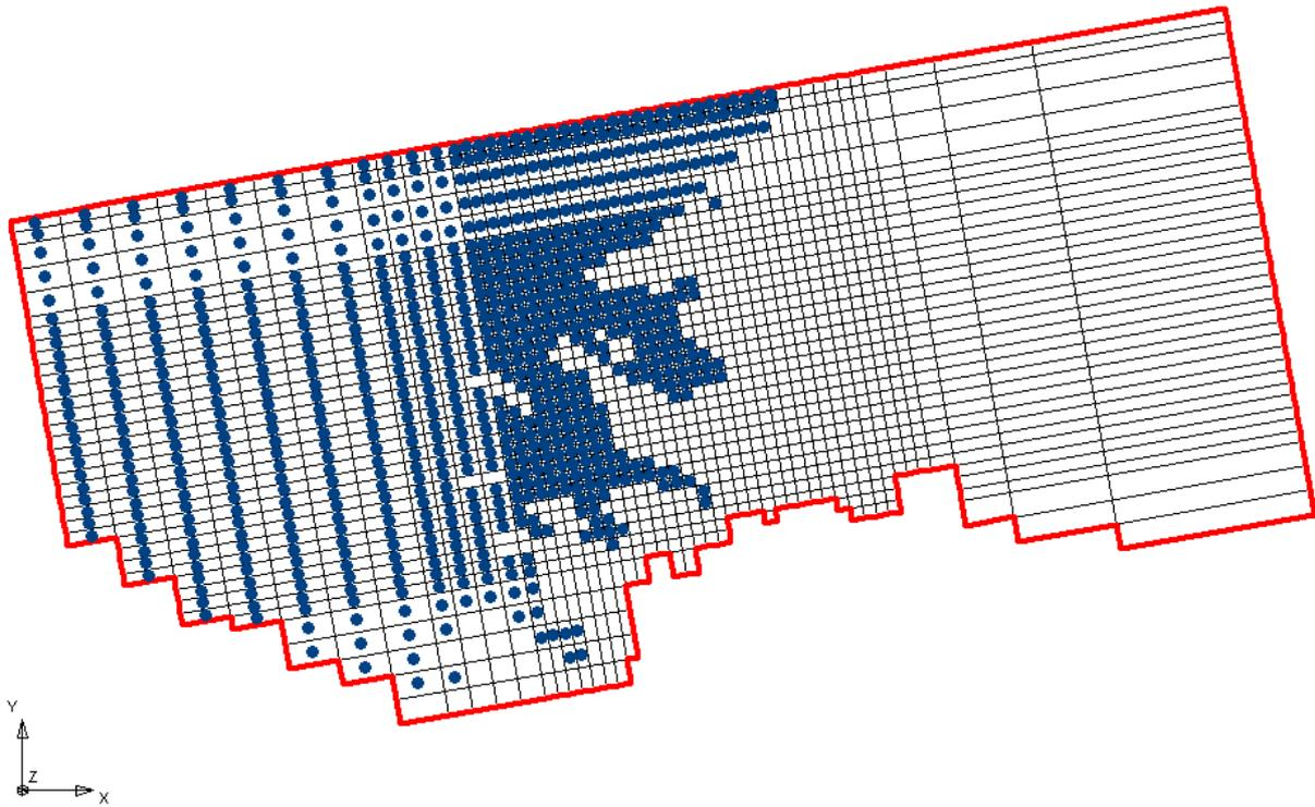
**Figure 4:** Configuration of rainfall recharge area over unconfined aquifer of the model.
