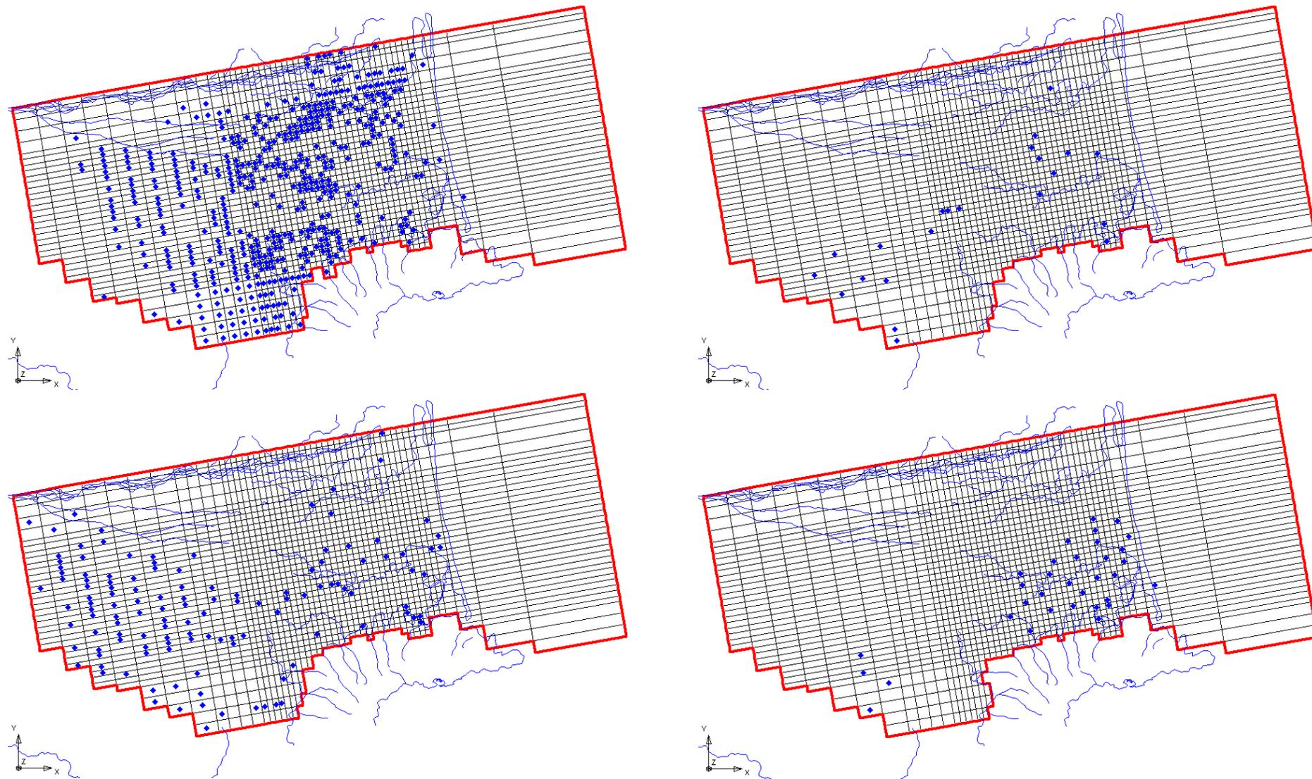
**Figure 6:** Distribution of well cells: layer 1 - upper-left, layer 2 – lower left, layer 3 – upper right, layer 4 – lower right, layer 5 – not shown (8 well cells only).
