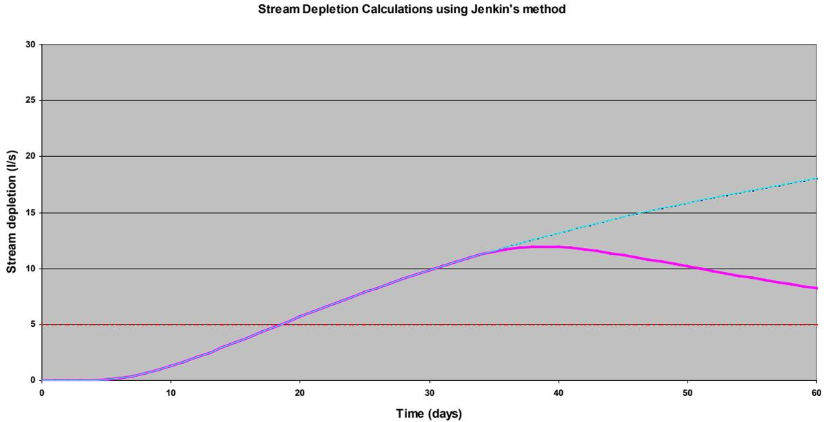
**Figure A2-1: Case 1 - Stream depletion effect for well with stream depletion factor of 100 days.**
