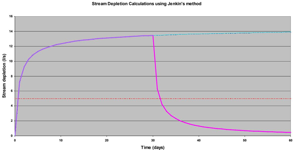
**Figure A2-2: Case 2 - Stream depletion effect for well with stream depletion factor of 1 day.**
