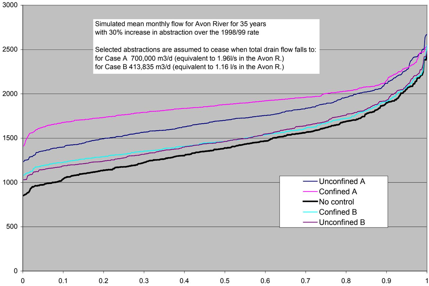
**Figure 10: Distribution of simulated Avon River baseflows for alternative restriction regimes.**
